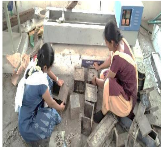
Figure 2 Concrete cube preparation
